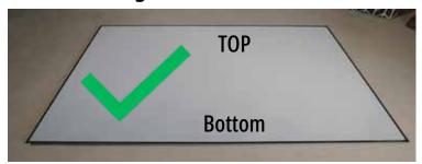
**CORRECT DIRECTION**: The material should have a white/gray color when viewed from an angle as shown below. This is how to distinguish the correct direction of the **REFLECTIVE LAYER** positioned at the bottom of the material's microstructure.
