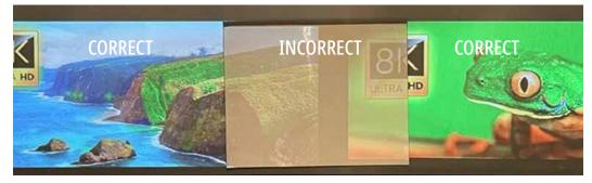
Example of screen hung up in the wrong direction with lights off. Projection may still look good but when Ceiling lights are turned on the image looks washed out. This is due to the material not absorbing overhead light.
